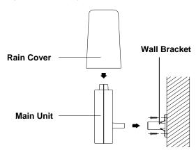
An ideal mounting place for the thermo-hygro sensor would be the outer wall beneath the extension of a roof, as this will protect the sensor from direct sunlight and other extreme weather conditions.
